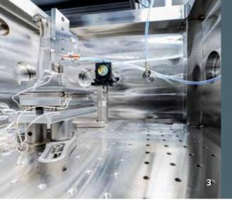
The laboratory at Fraunhofer ILT will be located next to the actual laser development laboratory and will offer a separate beam source. This allows experiments to be carried out in three different chambers in parallel. The opening at the end of 2019 will feature a source that has 500 watts, pulse energies up to 1 mJ and pulse durations below 100 fs, and will be scaled to 2.5 kW (5 mJ) by mid-2020. The metrology equipment includes an extensive range of beam diagnostic tools.
