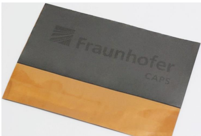
Image 1: Laser-structured anode material of a Li-ion battery. © Fraunhofer ILT, Aachen, Germany.
